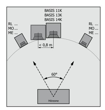
It is not necessary to place the subwoofers exactly in the middle of the stereo base, since locating the sound source below 100 Hz is only possible to a limited extent. But it should always be on the same level between both front systems. Placing the subwoofer outside the stereo base may result in unwanted localization of the BASIS 11K, BASIS 13K and BASIS 14K.
