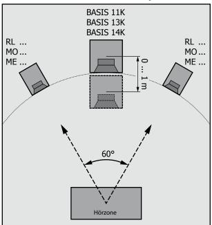
The distance of the BASIS11K, BASIS13K and BASIS14K should not exceed 1 m (3'3") in the direction of the listening zone to the plane of the front speakers. A range adjustment is provided for the devices in this range and can be made on the adjustment knob (2) (see the figure in chapter 6).
